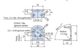
Burrs must extend less than 0.1 mm.
