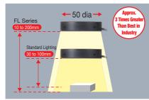
Because a large area in the field of view can be inspected, the installation location can be selected more flexibly.
